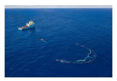
**Figure 2:** This image depicts the process of collecting the debris. Natural forces sweep the trash into the barrier that because of the anchor moves slowly and captures them all. 12
